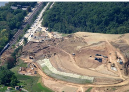
A photo of a landslide in Kilbuck Township that occurred during development preparations on a slide-prone slope. Photo courtesy of DEP.
